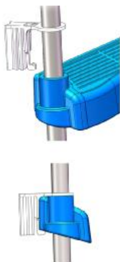
STEP II: Diagram of Bushings installation
