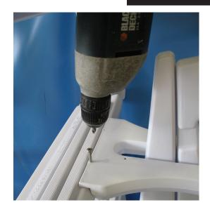
Screw Upper Brace of Entrapment Barrier into the third step of the Inside Portion of the Ladder with (2) #10 x 1-1/4" screws.
