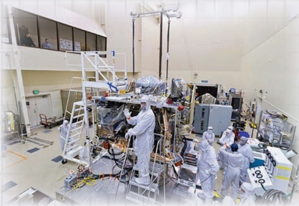
The OSIRIS-REx spacecraft with the Sample Acquisition and Return Assembly (SARA) being installed.
