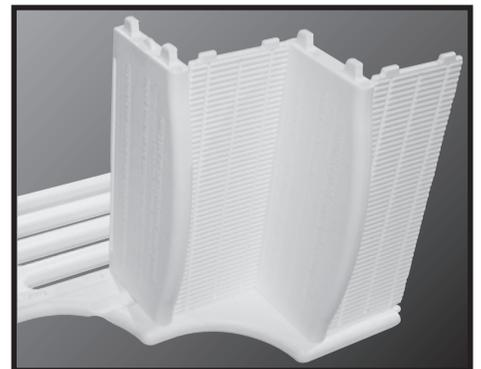
**#4:** Place a tread into the slots and over the riser. With a rubber mallet tap tread down until locked into place.
