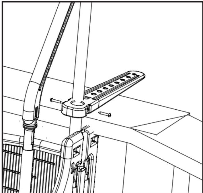
**#3:** If step is being used with pool deck rotate the two deck connectors to sit on to pool deck and attach using two #10 x 1-1/4" self tapping screws in each connector.
