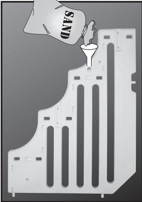
**#1:** Using a funnel pour 25 lbs. of dry play sand into each side panel. Shake the panel to settle sand to the bottom. Cap the fill holes using the two white push plugs from the hardware bag.
