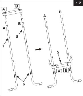
**IMPORTANT:** Ensure the J-shaped legs are pointing outwards before installing the steps.
