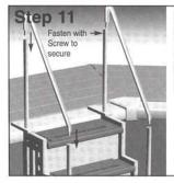
Spray the ends of the handrails with silicone or liquid soap and slip the ends of the handrails into the open ends of the posts until they are fully seated. Secure in place using one #10x1-1/4" screw per post.
