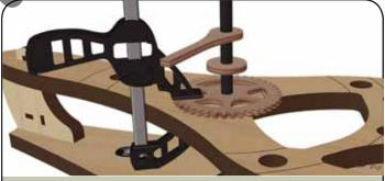
Press the Hour Hand Spacer (AU) and Hour 5. Hand (BQ) onto the Hour Gear(AT).
