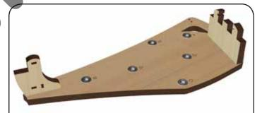
The bearing flanges must lie flat against the 5. Rear Frame (BA).
