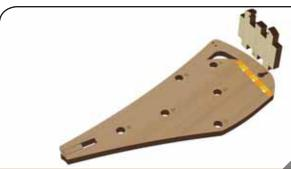
Glue the Upper Frame Spacer (BE) to the 2. marked side of the Rear Frame (BA)
