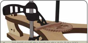
DO NOT GLUE the parts to the Axle Tube (CE) 6.
