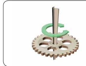
4. To sand holes and smaller openings, tear a small strip of sandpaper and tightly roll it into a cone shape small enough to fit. Work the sandpaper into the opening, twirling it as it is moved in and out.
