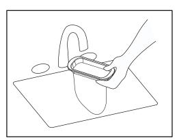
MARNING: Using your cleaner without the filter bag/seal in place will cause blockages in your machine and void vour warrantv.
