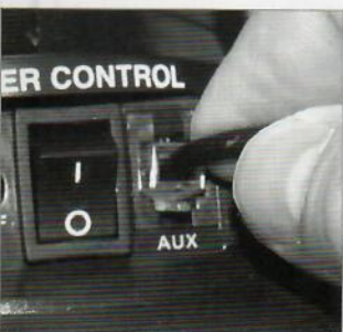
Fig. 7: For users NOT USING #497 Autostar: Plug one end of a connector into the AUX port of your telescope's computer control panel.
