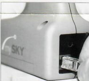
Fig. 5: Plug 4 pin connector into mySKY.
