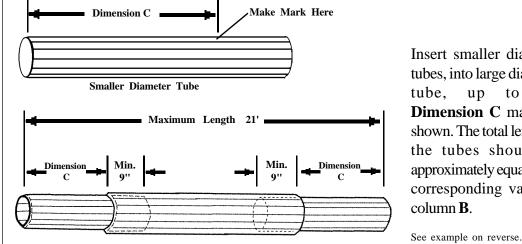
Insert smaller diameter tubes, into large diameter tube, up to the **Dimension** C mark, as shown. The total length of the tubes should be approximately equal to the corresponding value in column **B**.
